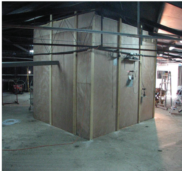
Fig. 3. Left: A photo of the fog chamber. Right: The set of sprinklers constructed near the fog chamber's ceiling.
