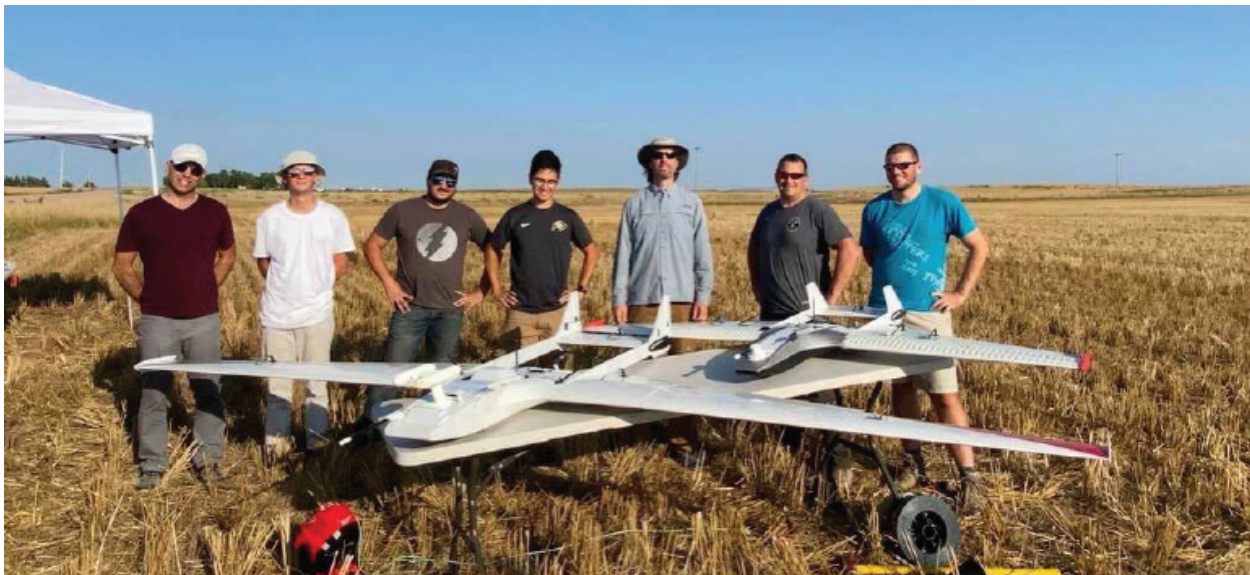
Fig. 2. The two Uncrewed Aircraft Systems used for the research project UAS (Seed) is on the right side and UAS (Obs) is on the left side of the figure. The flight crew with ad hoc team members shown. Photo courtesy of Alex Hirst.
